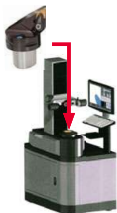
Measurement outside the machine
