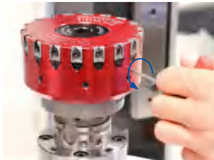
1. Turn the threaded spindle one turn anticlockwise with a hex-wrench, width across flats 2.5.
